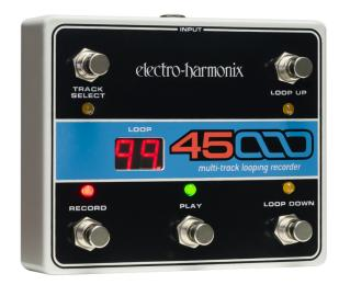
It makes everything faster and easier by delivering hands free operation of key functions. Choose a new track or loop without missing a beat. Get instant access to up to 100 loops per SDHC card. The Foot Controller receives power from the 45000 and connects to it with a standard mono guitar cable. It's a must have!
